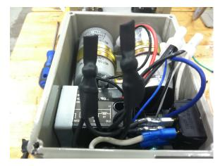
STEP 3: Install new power cord- Connect the green wire to ground, connect the brown wire on the bottom of the switch, and connect the blue wire on the top of the switch.
