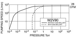
The FluidX W2V80 rotary vane vacuum pump features a rugged, twostage, air-cooled design and is capable of pumping speeds of 28 cfm and producing an ultimate vacuum of 10-3 Torr. Lightweight, quiet, and compact, the W2V80 features an anti-suckback and gas ballast valve, quick disconnect ISO/KF fittings, and is ideal for a variety of applications.
