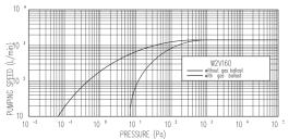
The FluidX W2V160 rotary vane vacuum pump features a rugged, twostage, air-cooled design and is capable of pumping speeds of 56.5 cfm and producing an ultimate vacuum of 10-3 Torr. Lightweight, quiet, and compact, the W2V160 features an anti-suckback and gas ballast valve, quick disconnect ISO/KF fittings, and is ideal for a variety of applications.
